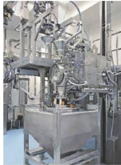
A Hammerwitt-6 with a Profi-Valve 150 dosing device mounted at the inlet is used at the Irish pharmaceutical manufacturing plant
